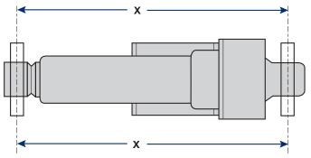
Mounting pins must be parallel to each other as shown above. Pins which are not parallel can cause excess vibration or actuator binding.
