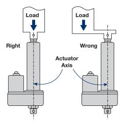
Loads should act along the axis of the actuator. Off-center loads may cause binding and lead to premature unit failure.
